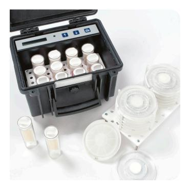
The Lovibond<sup>®</sup> DI10 Incubator is designed for the reliable incubation of bacteriological slides, on-site, in a laboratory or even while mobile in a car or van.
